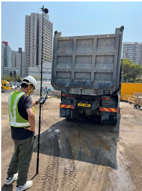
Figure 1 Photo of noise measurement (1)
